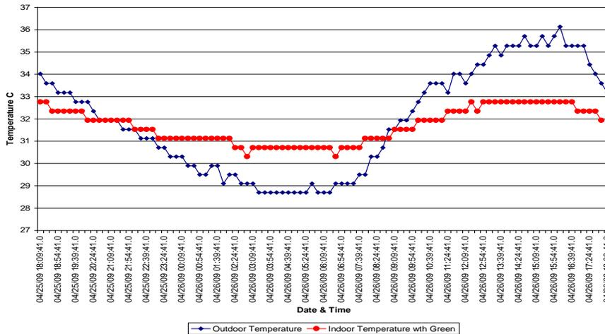
**Figure 3:** Profile of outdoor air temperature and indoor air temperature with green roof and bare roof. (Source: Author)
