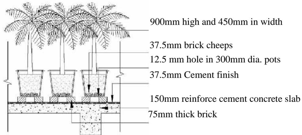
**Figure 2:** Section of construction of the green roof top (Source: Author)
